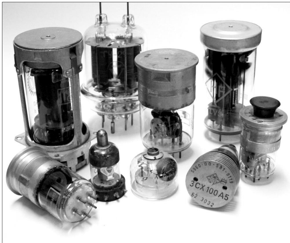
Obr. 2 - Elektronky pro VKV a mikrovlny 1939-1980 UHF and microwave tubes (1939 - 1980)
