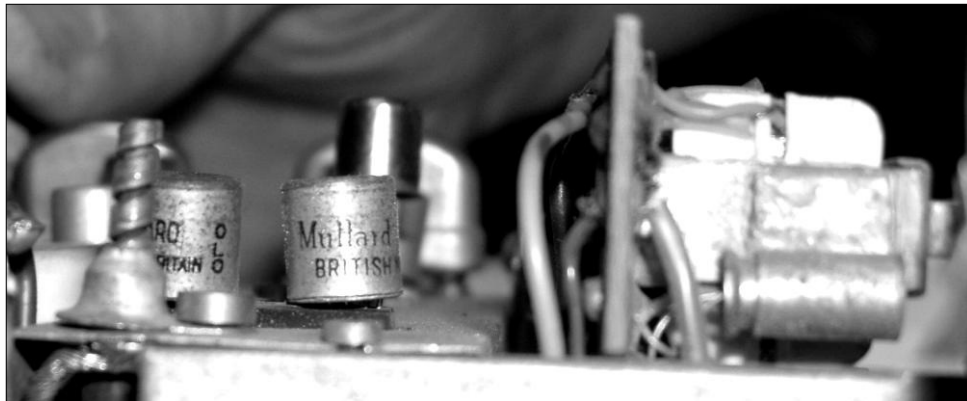
Obr. 3 - Detail PA (QRP) se dvěma tranzistory OC171 pro 2 m (1963) Detail of PA (QRP) with 2x OC171 transistors for the 2-m band (1963)
