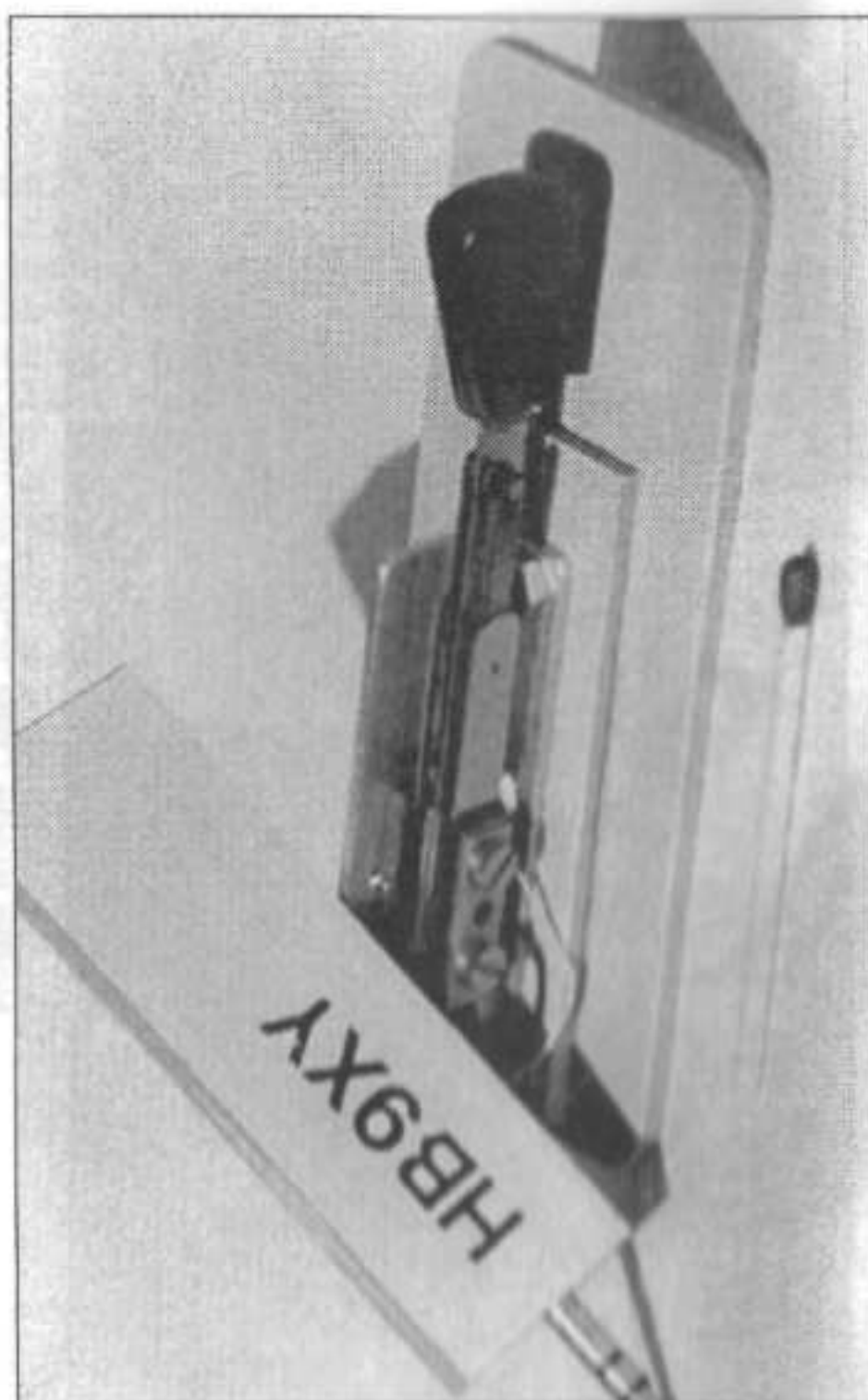
Mini paddle made of relay parts
